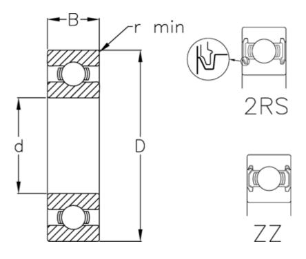
B = 9 d = 10 D = 28 Dynamic load C (kN) = 5.1 Max rpm greased = 25000 Max rpm oil lubricated = 30000 r min = 0.6 Static load C0 (kN) = 2.39
